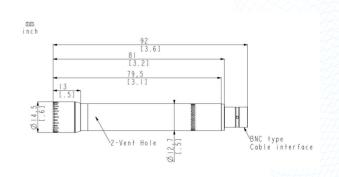
Fig.2 CRY3213 NVH Ruggedized Measurement Microphone Drawings
